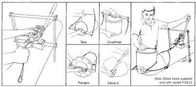
The lightweight PULLER-CLAMP is easy to transport and assemble. This makes the unit very practical for close work in a trench or high up on a pipe rack.
